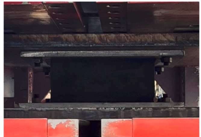
Fig. 10. Vertical compression test (10 MPa).
