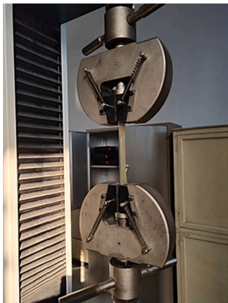
Fig. 2. Tensile test of the FRP.
