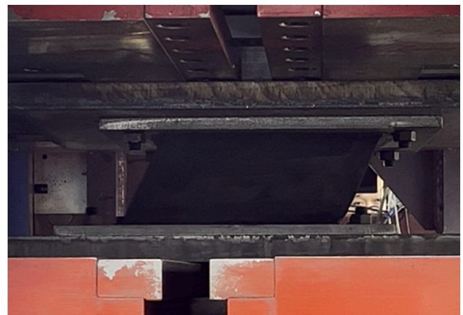
Fig. 11. Horizontal shear test (5 MPa-100% \gamma ).
