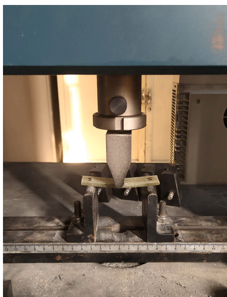
Fig. 5. Bending test of the FRP.
